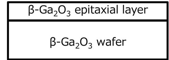
Cross section of β-Ga<sub>2</sub>O<sub>3</sub> epitaxial wafer
